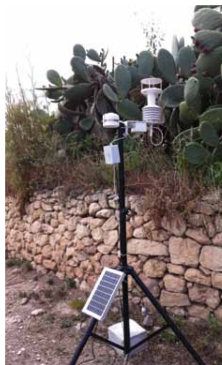
Above: the Envirologger set in position on the Tarxien site gathers a range of useful data
